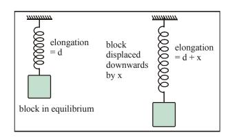
• Mean position : spring in elongated by  $d = \frac{mg}{k}$
