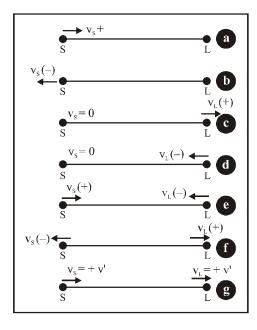
$$v' = \frac{\left(v - v_L\right)}{v}v \quad \text{i.e. } v' < v$$
