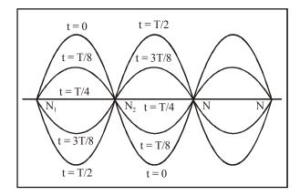
• It is clear from the figure that since nodes are, at rest they don't transfer energy. In a stationary wave, energy is not transferred from one point to the other.
