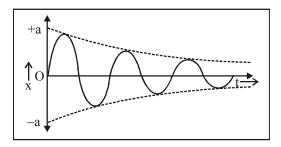
(iii) Due to decrease in amplitude the energy of the oscillator also goes on decreasing exponentially.
