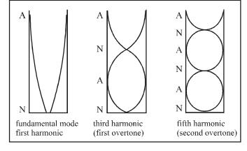
• There are only odd harmonics in a tube closed at one end.
